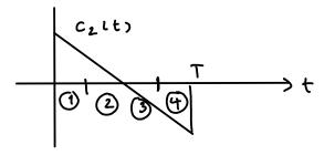
To ensure orthogonality, we must have sections (1) and (4) multiplied by the same sign and sections (2) and (3) multiplied by the same sign.
