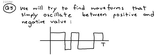
Now, to make it orthogonal to C.(t), the positive portion of the graph must be equal to the negative portion of the graph. (So, the above waveform doe, not work.)
